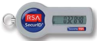
Fig. 1 – RSA SecurID key fob
